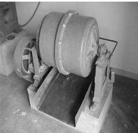
Figure 3: A sample ball mill.
