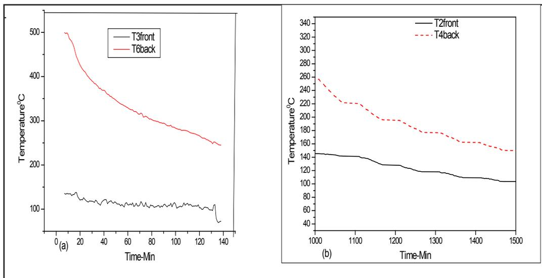
Figure. 4: Temperature distribution in the incinerator
