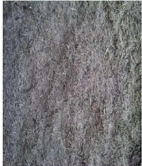
Figure 2: RHA after combustion
