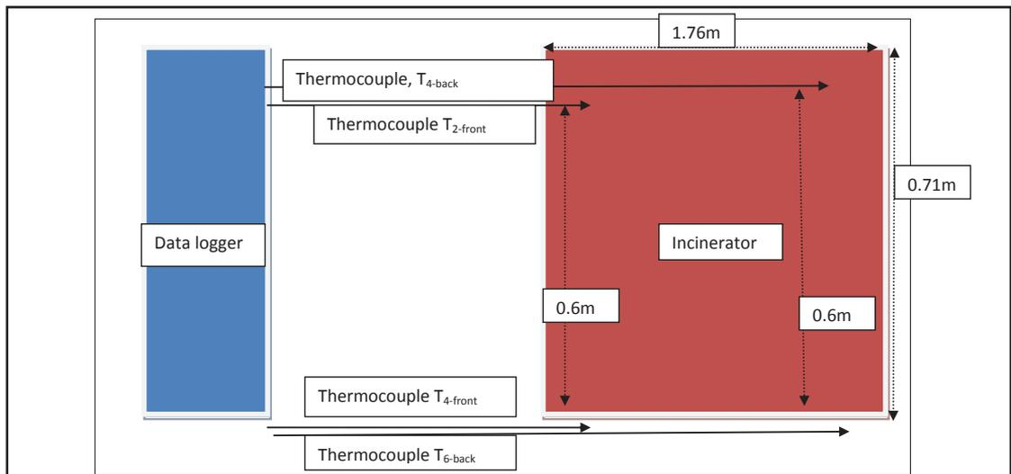
Figure.1: Schematic drawing of thermocouple positions inside the incinerator
