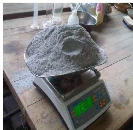
Figure 4: Sample of RHA after grinding
